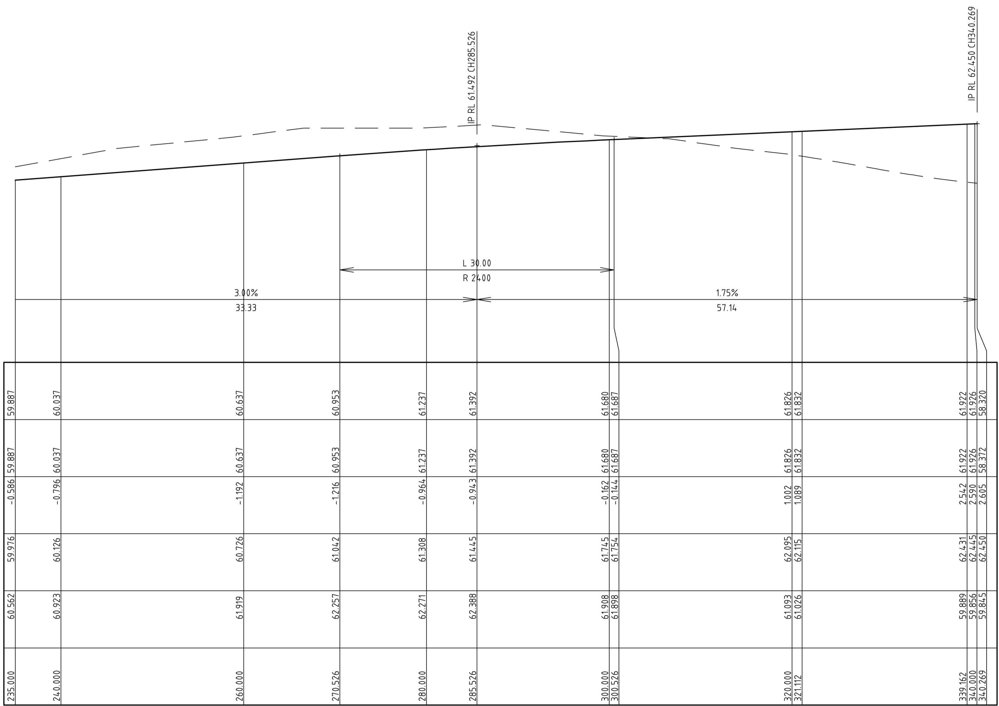
LONGITUDINAL SECTION - ROAD 6 SCALE HORIZONTAL 1 : 250 VERTICAL 1 : 100
