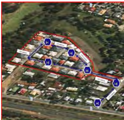
Figure 6 – Hydrant System design to minimum standards
